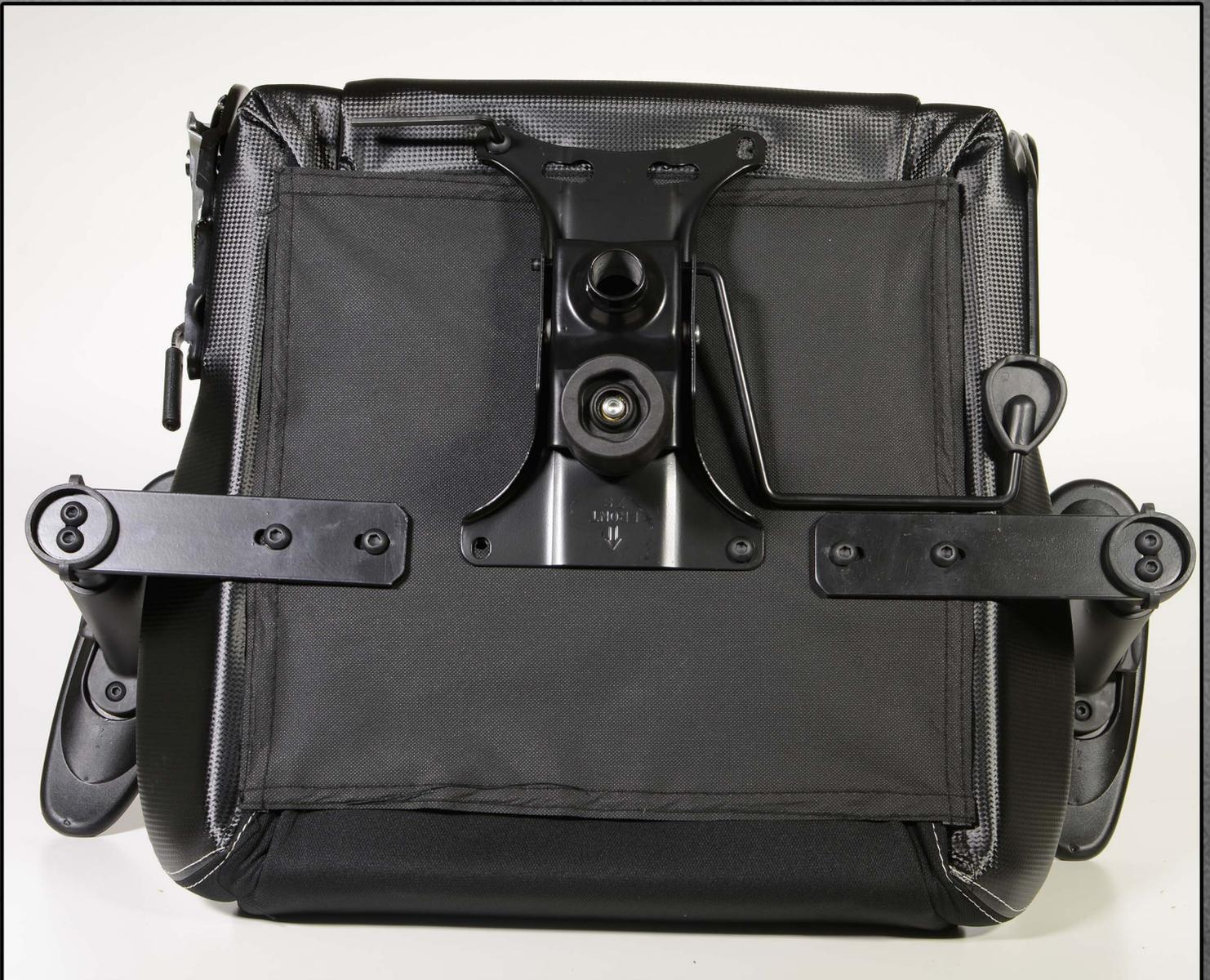
Flip the chair and attach the backplate as shown in the picture above. Make sure the text and arrow that says "FRONT" are facing the right way. Attach two of the screws loosely, this can be done by hand. When it is fitted correctly, attach the last two screws and tighten.
