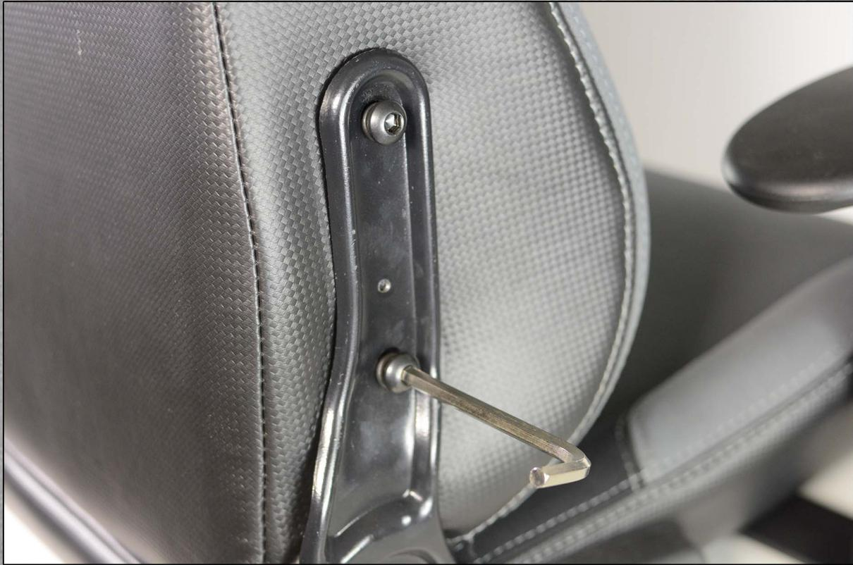
Fit the backrest on top of the seat, insert and screw loosely.
