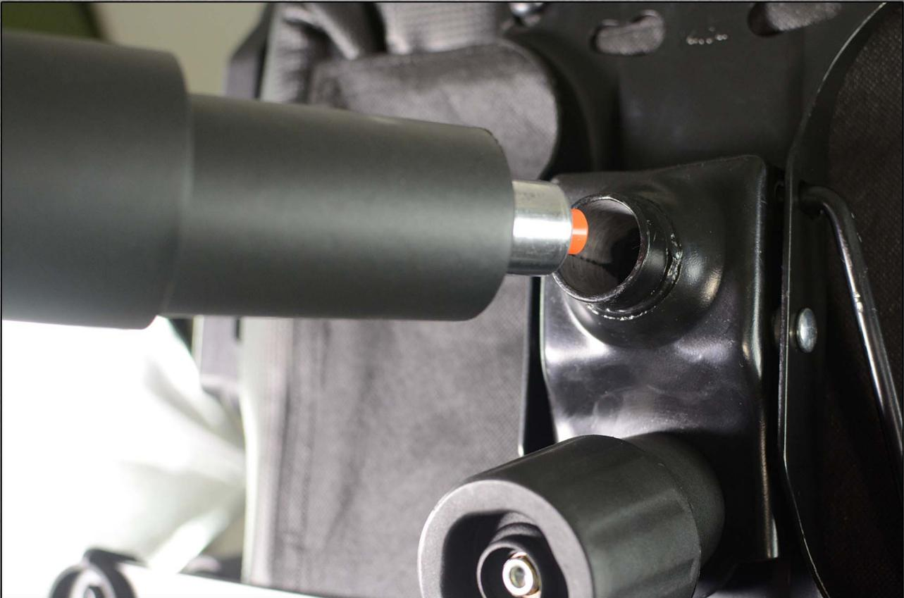
Insert the gaslift into the backplate like above.
