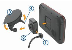
2 Press the mount (2) onto the suction cup (3) until it snaps into place.
