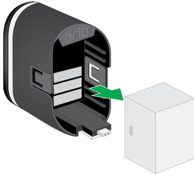
4. Align the battery and insert it into the battery compartment.
