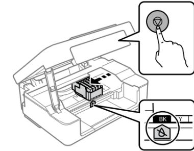
**!** Never touch the ink cartridges while the ink cartridge holder is moving.
