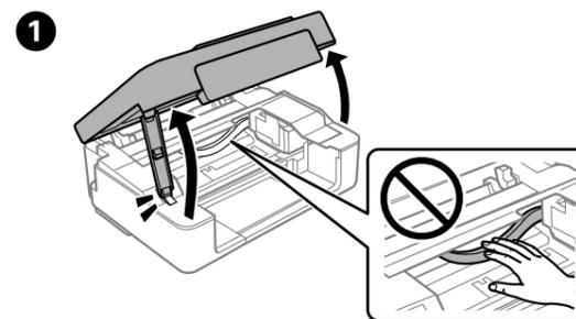
**2** Press to move the ink cartridge holder. It stops at the mark to indicate an expended or low-ink cartridge.
