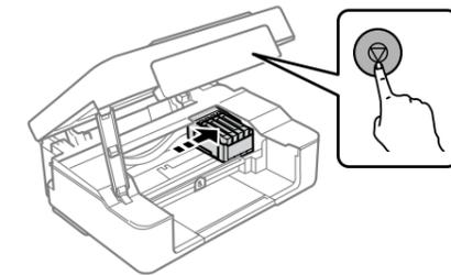
**!** If there is another expended or low-ink-level cartridge, the ink cartridge holder stops to indicate the cartridge with the mark. Press repeatedly until it moves to the replacement position.
