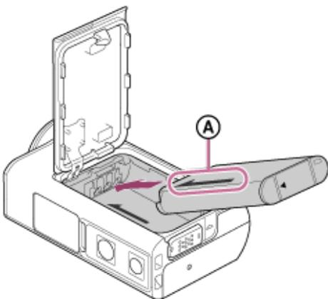
**A** : Align the direction of the arrow on the camera and the battery pack.
