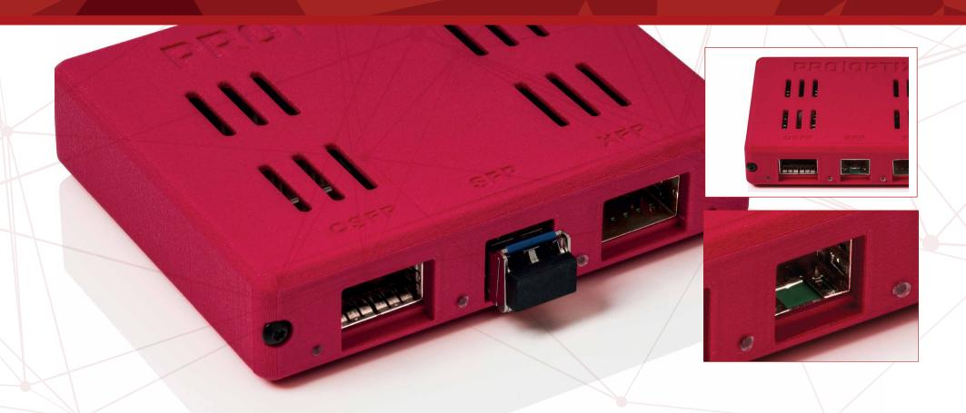
Pro Optix Pro Coder is used for transcoding transceivers and changing channel on tunable DWDM. It is suitable for data centers and networks as it gives installers and technicians a field of incredible flexibility – transceivers can be re-encoded according to the current needs. It also gives the possibility of remote support and access. Pro Coder is easy to use and fits into several form factors and can be recoded to many different brands.
