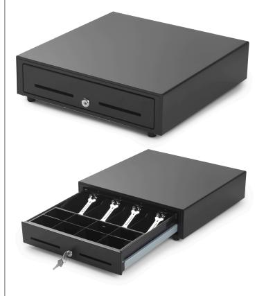
SPECIFICATIONS **Materials** Metal and steel. **Bill Trav** Four metal bill clips. **Coin Tray** Removable two-row tray with eight compartments. Media Slot Front access slot for fx checs and credit card receipts. Lock 3-position Key Lock. **Micro Switch** Open by driver signal to the solenoid. I/O Interface 12V/24V for RJ11/RJ12. Durability One million operations. Color Black.
