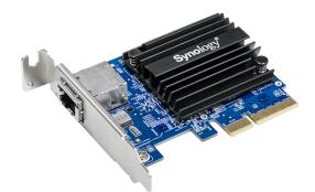
Equipped with an RJ-45 connector and supports IEEE 802.3an/bz (10GBASE-T/NBASE-T) and 802.3x, E10G18-T1 helps you smoothly migrate to a 10GbE networking environment with your existing infrastructure. Supporting backward compatibility and auto-negotiation between 10Gbps, 5Gbps, 2.5Gbps, 1Gbps and 100Mbps data rate, E10G18-T1 is an economic solution to overcome the data transmission bottleneck for small businesses and home users.
