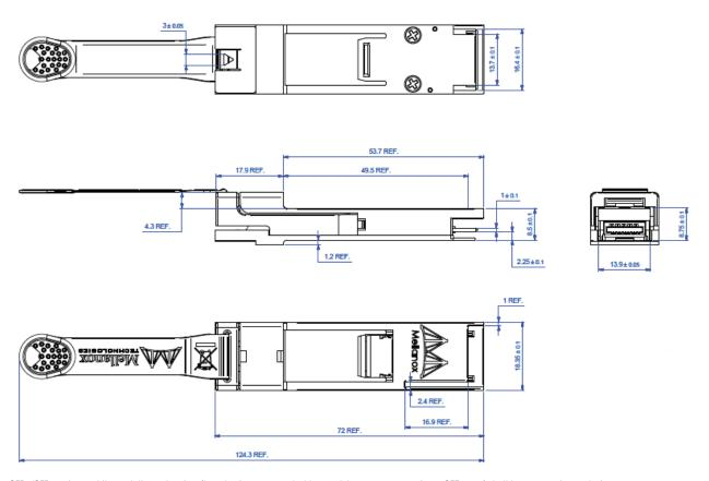
Note: The SFP+/SFP mating paddle card dimension A10 (length of component/solder mask keep-out area, refer to SFF-8071) shall be >6.0mm instead of >5.5mm. The reason for this requirement is to prevent damaging the adapter when trying to insert an SFP upside down.
