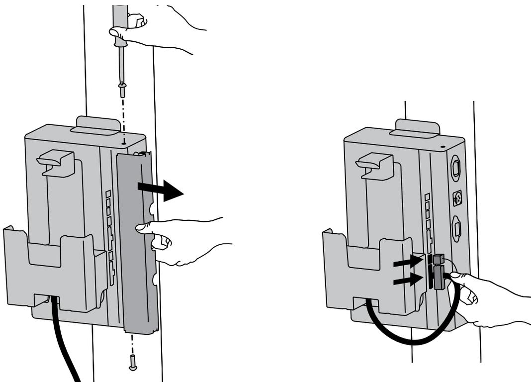
**7 a** Attach SOCI to worksurface, then route cable down and plug into power module.
