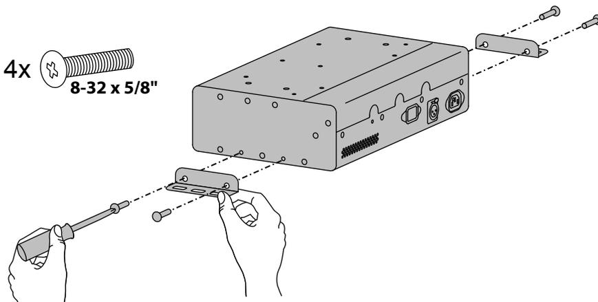
**2** a. Remove these four screws from the power module.
