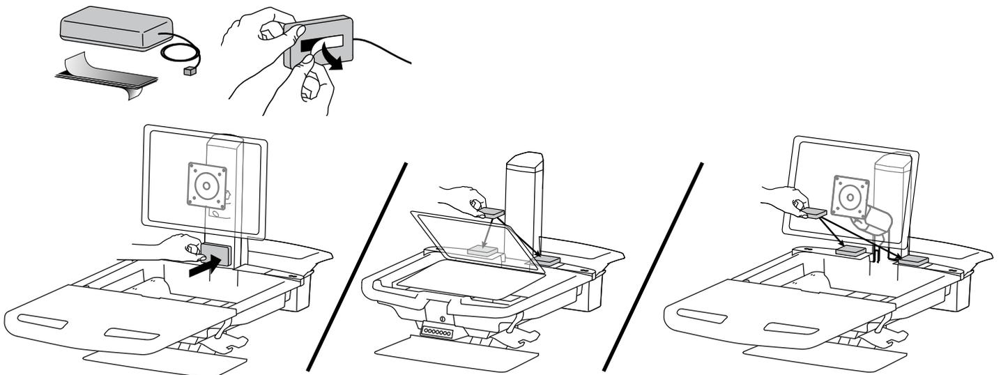
**b** Route SOCI cable down through bottom of enclosure and plug into power module.
