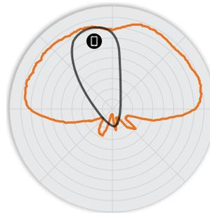
Figure 5. T610o 5GHz Elevation Antenna Patterns
