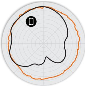
Figure 3. T610o 5GHz Azimuth Antenna Patterns
