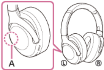
A: Location of the built-in antenna
