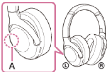
A: Location of the built-in antenna
