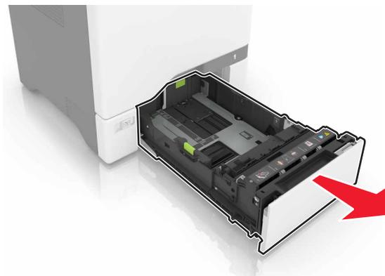
**2** Remove the separator bracket.
