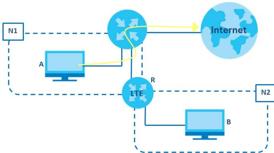
You need to specify a static routing rule on the LTE7460-M608 to specify **R** as the router in charge of forwarding traffic to **N2**. In this case, the LTE7460-M608 routes traffic from **A** to **R** and then **R** routes the traffic to **B**.
