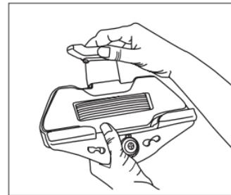
3. Insert tablet into the headrest mount base, then place the top of the cradle over the tablet.
