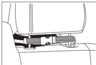
6. Please hold the tablet during the following removal process to ensure it does not fall. To remove the tablet, pull the Boa® knob out to release the cable tension and then pull the top of the cradle away from tablet. Remove tablet.
