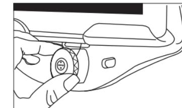
7. To store the holder, place the top of the cradle back onto the main holder, then push Boa® knob in and turn clockwise until cable is tightened.
