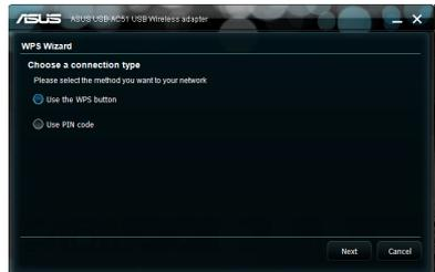
3. Press the WPS button on the AP or station to establish a secure connection.
