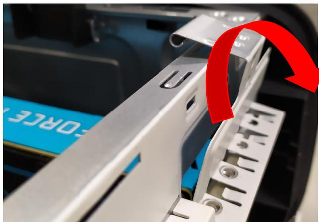
5. Release the latch that secures the graphic board to the mainboard.
