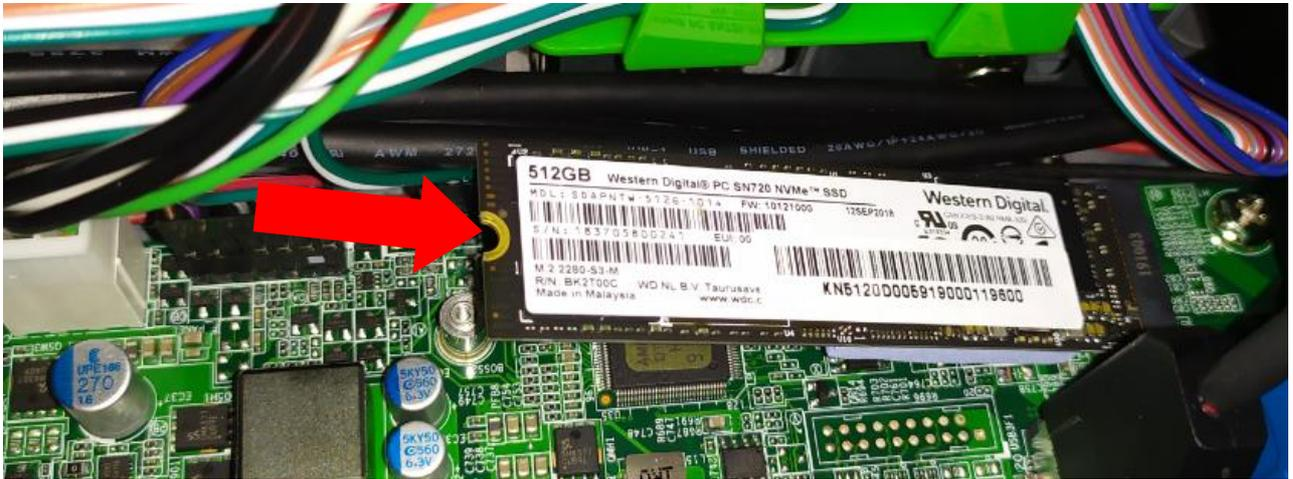
3. Secure the M.2 SSD module and mainboard with screws.
