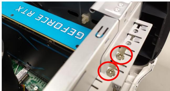
4. Unlatch the metal clip that secure the graphics board to the chassis.
