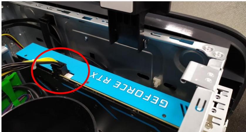
3. Remove the screw that secure the Graphic boards to the chassis.
