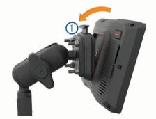
2 Push the top of the device forward until it snaps into place. The latch ① on the mount stays up after you insert the device.
