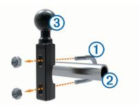
2 Tighten the nuts to secure the base. NOTE: The recommended torque is 50 lbf-in (5.65 N-m). Do not exceed torque of 80 lbf-in (9.04 N-m).
