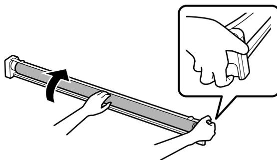
While holding down the take-up button, turn the basket by hand in the direction indicated by the arrow. After turning it all the way, draw out the basket.
