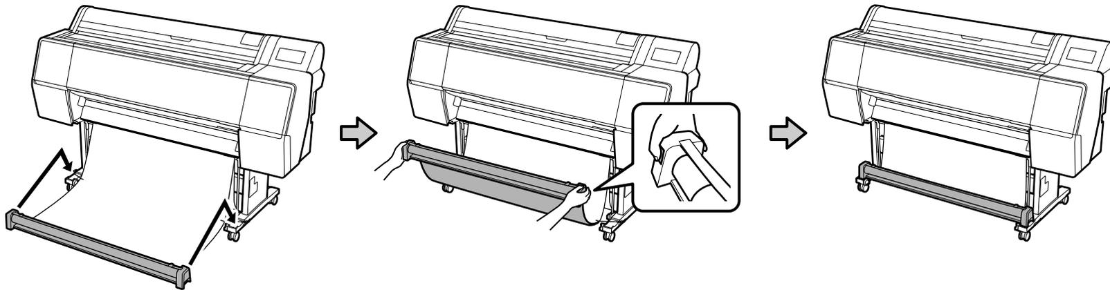
**Removing protective material**
