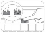
The camera button is connected to the water drainage hole on the back of your MateBook 14. If you accidentally spill water onto the camera, it will drain out from the drainage hole.
