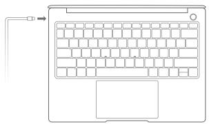
Your MateBook 14 has a built-in rechargeable battery, and you can charge it using the adapter and USB-C charging cable that came with it. The indicator blinks white during charging.
