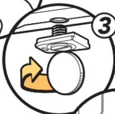
3 Using a coin, screw the clip into your camera.
