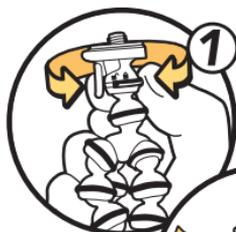
1 Rotate the rubber ring counter clock-wise to lock the button and clock-wise to unlock. 🔒
