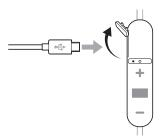
It takes up to 2 hours to fully charge the headphones from a completely drained battery state. While charging, the indicator light is red and turns off once charging is complete.
