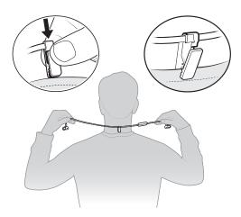
2 Another option for improving fit and stability is to cinch the excess cord up into a loop with the clip instead of attaching it to your clothing.
