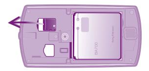
Remove the battery cover, then draw the memory card outward to remove it.
