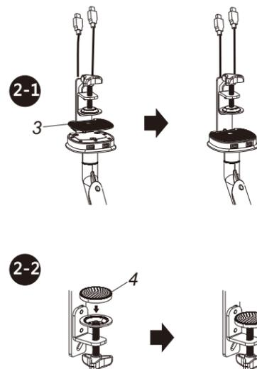
select proper position according to thickness of desk
