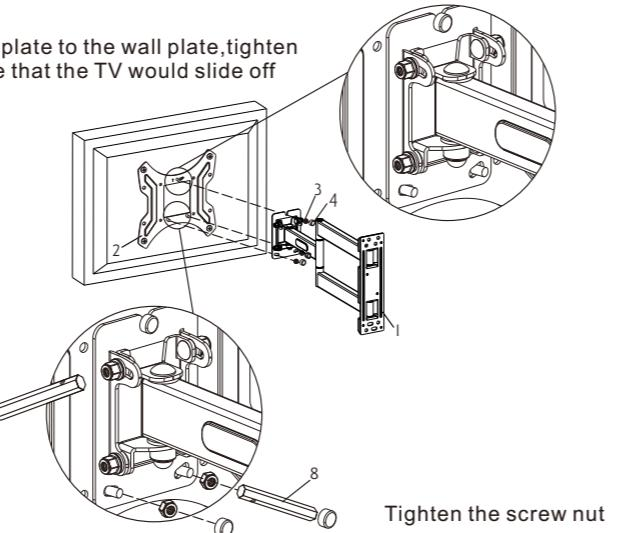
Tighten the screw nut
