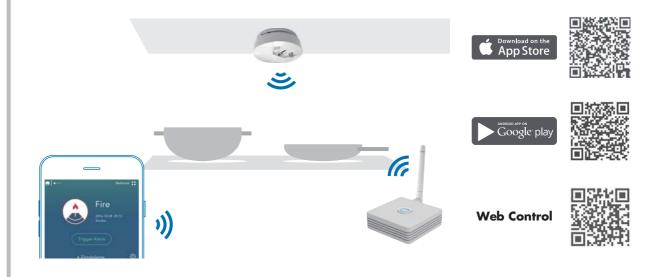
Receive the alarm if smoke or heat detected
