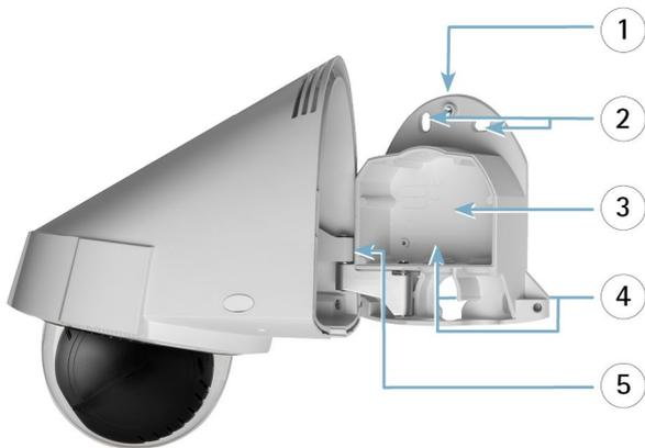
An AXIS P54 camera comes with a built-in wall bracket (1) for easy installation. Oblong screw holes (2) make leveling easier. Extra space (3) is provided for service loops and there are holes (4) for cables. With a lift-off hinge (5), the camera, together with the integrated sunshield, is easily hung onto the wall bracket, freeing up hands to make cable connections. The hinge allows the camera unit to swing in and be fastened with three screws.
