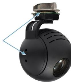
An AXIS P54 camera is directly attached to the drive shaft of two motors (pointed out in image at left)—one for panning and another for tilting the camera. With no parts such as belts or gears, AXIS P54's durable pan/tilt system is fast and provides customers with a reliable, low-maintenance PTZ camera.
