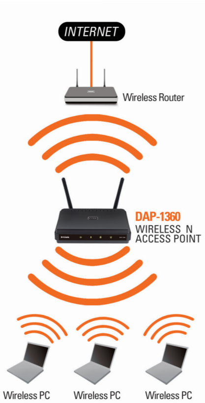
Extending the Wireless Coverage of a Wireless Router Using the DAP-1360
