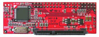
Convert High Capacity SATA Hard Drive and SATA Storage Device to operate with IDE Host Controller!
