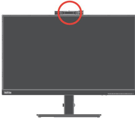
Slide the camera shutter open or close to enable/disable the camera.
