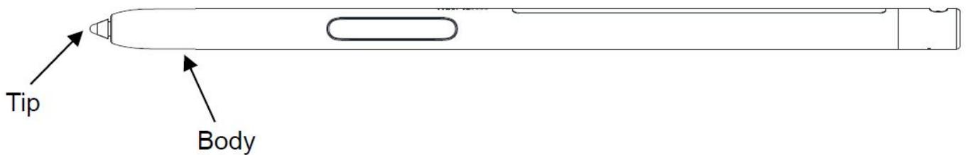
2. Push in a brand-new tip with fingers until the tip bottoms out in the hole.
