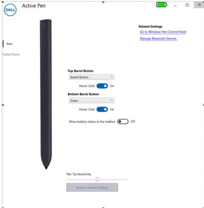
1. **Top barrel button:** Top barrel button can be disabled or programmed to run specific applications or functions as listed below:
