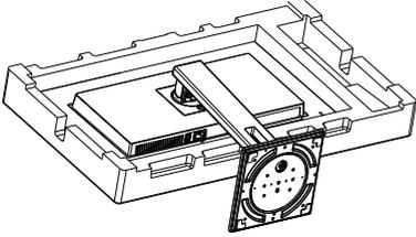
2. While keeping the release button pressed, tilt the base and slide it out.
