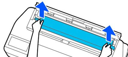
**6** Detach the transparent flange from the spindle.
