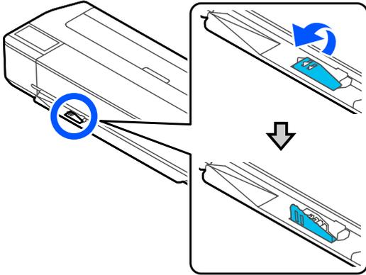
Leave the support lowered when printing to a size other than equivalent to B1 width.
