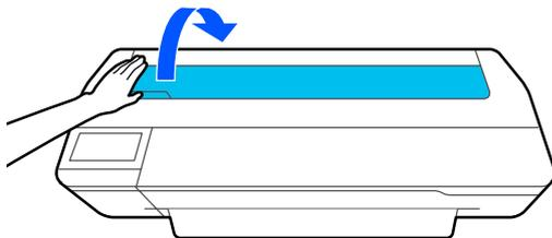
**3** Unlock the center lock and open the roll paper cover.
