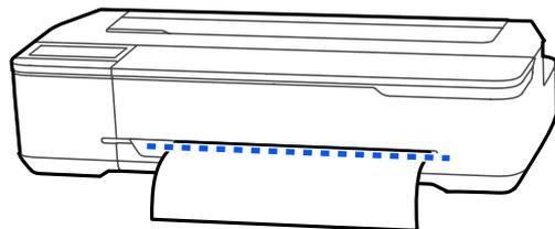
Cut lines cannot be printed further inside than the bottom margin. Once you have finished moving the paper, touch
