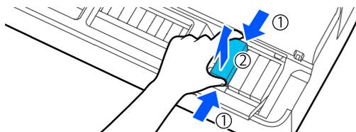
After ink discharge, reinstall the ink cartridges. Place the removed ink cartridges nearby with the ink supply port down, or laid horizontally.
