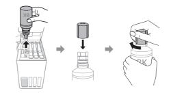
**Note:** Do not leave the ink bottle inserted; otherwise the bottle may be damaged or ink may leak.
