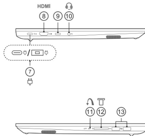
Note: The power connector (7) varies by model. Ports labeled with can charge connected devices when the computer is powered off.
