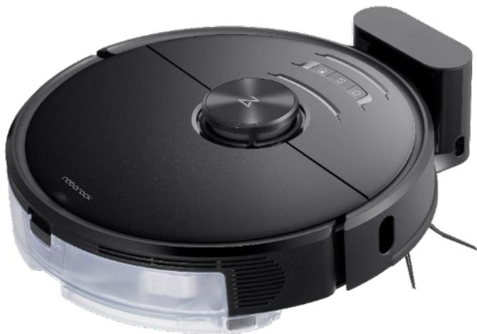
When cleaning large spaces, Smart Top-up allows S6 MaxV to return to the dock when power is low, and recharge just enough to finish the clean.
