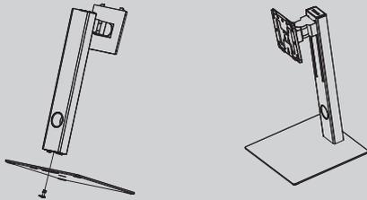
4. Insert the hook at the front end of the lifting bracket shaft diagonally into the rear shell bayonet, and gently press the tail end perpendicular to the surface of the rear shell, so that the lock of the lifting bracket can be buckled to the quick release button of the rear shell, and the quick release button has a return. The bounce action means that the tail end has also been stuck in place.
