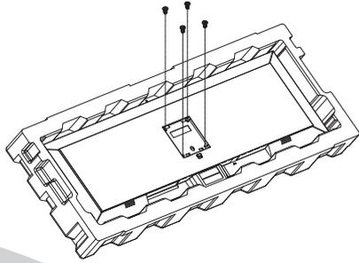
2. Find 4 (M4\*9) studs from the accessories, lock them in the threaded holes of the bracket, and lock them with a flat-blade screwdriver.
