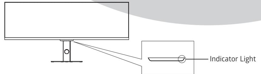
Solid blue light indicates power is on and the monitor is operating normally. Flashing blue light indicates no video source, no horizontal or vertical signal has been detected or power is low. Please ensure your computer is on and all video cables are fully inserted and/or connected.
