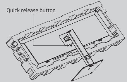
5. Grasp the bracket with your hands to stand up the machine. (note: during the process of erecting the machine, the machine is still in the lower styrofoam without taking it out, please do not pinch the screen directly with your hands to prevent the screen from breaking)
