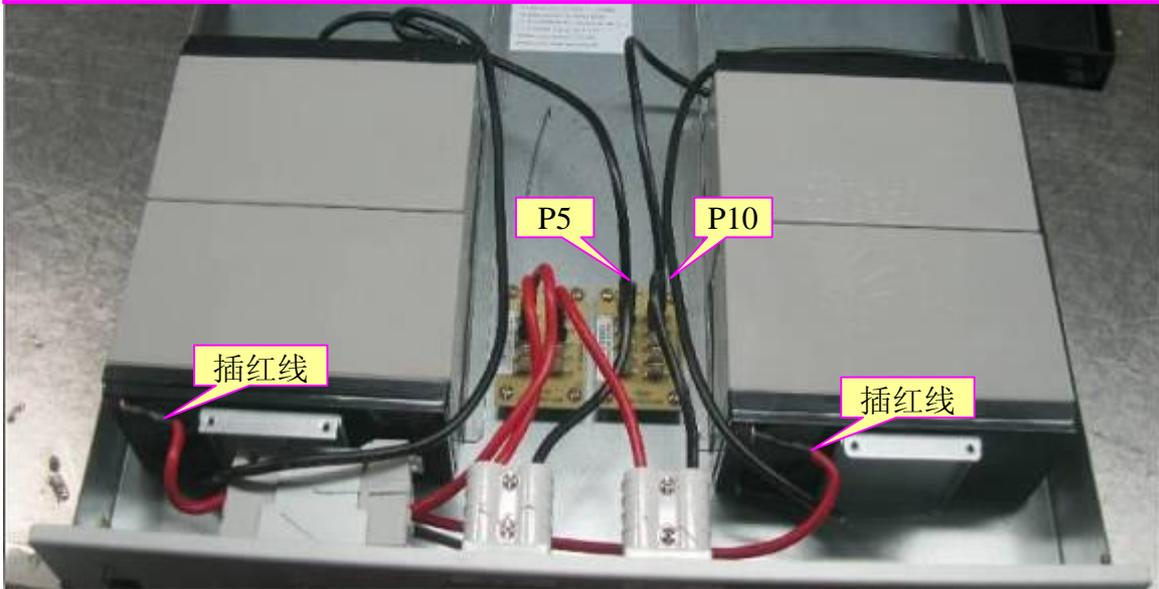
2、 As below shown, lock the baffle of battery on the base. Screw: **38-000008 - XXG \* 4**; Torque: **8 KGF - CM**
