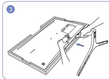
Place the protective Styrofoam (cushion) included in the package on the floor and place the product facing down on the Styrofoam, as shown in the image. If Styrofoam is unavailable, use a thick sitting mat. Hold the back of the monitor as shown in the figure. Push the assembled stand into the main body in the direction of the arrow as shown in the figure.
