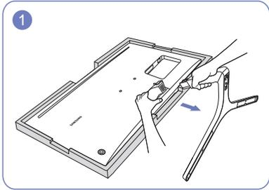
Place the protective Styrofoam (cushion) included in the package on the floor and place the product facing down on the Styrofoam, as shown in the image. If Styrofoam is unavailable, use a thick sitting mat. While holding the monitor with one hand, pull the stand neck with your other hand to detach the stand as shown in the figure.
