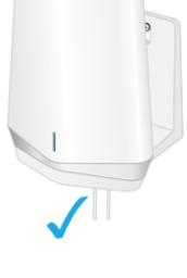
**Note:** When the screws are placed correctly, the holes at the back of the mounting bracket fit over the protruding screws, allowing you to slide the mounting bracket downward until the tops of the slots are resting on the screws.
