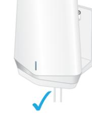
**Note:** When the screws are placed correctly, the holes at the back of the mounting bracket fit over the protruding screws, allowing you to slide the mounting bracket downward until the tops of the slots are resting on the screws.
