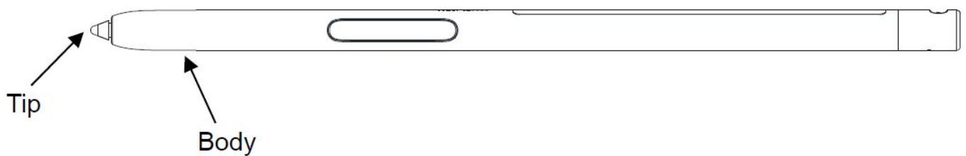
2. Push in a brand-new tip with fingers until the tip bottoms out in the hole.
