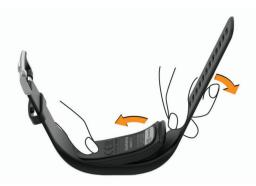
**2** Insert the device into the band, and stretch the band material around the device.
