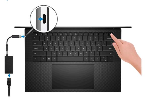
i NOTE: The battery may go into power-saving mode during shipment to conserve charge on the battery. Ensure that the power adapter is connected to your computer when it is turned on for the first time.
