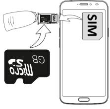
2. Place the SIM card into the correct tray slot to ensure that it can be recognized by the phone.
