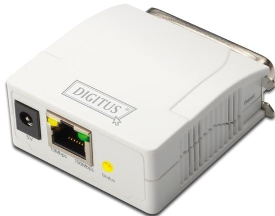
**Parallel Print Server, 1-Port 1x RJ45, 1x DB-36-pin male Centronics**
