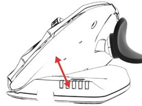
Adjust tilt for your desired mousing angle.
