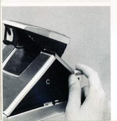
Put your thumb behind the shutter, without touching the bellows (C), and put your index finger on the focus wheel, as shown.
