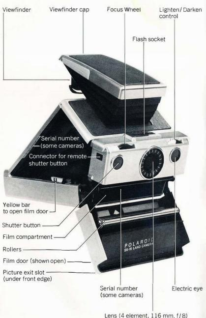
The film pack provides ten 3½ x 3½ inch pictures. In each pack is a flat battery to supply power for pictures made with that pack.
