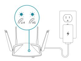
2 / Connect your computer to the Wi-Fi details printed on the Quick Installation Card. Type **http://dlinkrouter.local./** into a web browser. The default login password is "**password**". Follow the onscreen instructions to complete the setup.
