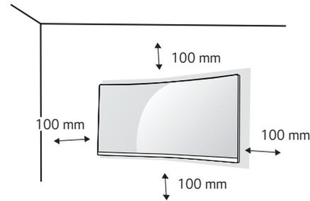
To install the monitor to a wall, attach a wall mounting bracket (optional) to the back of the monitor.
