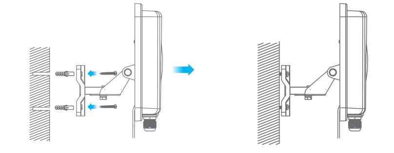
③ Insert nylon wall plugs into the wall. Use mounting screws to secure the main frame to the wall through the nylon plugs.
