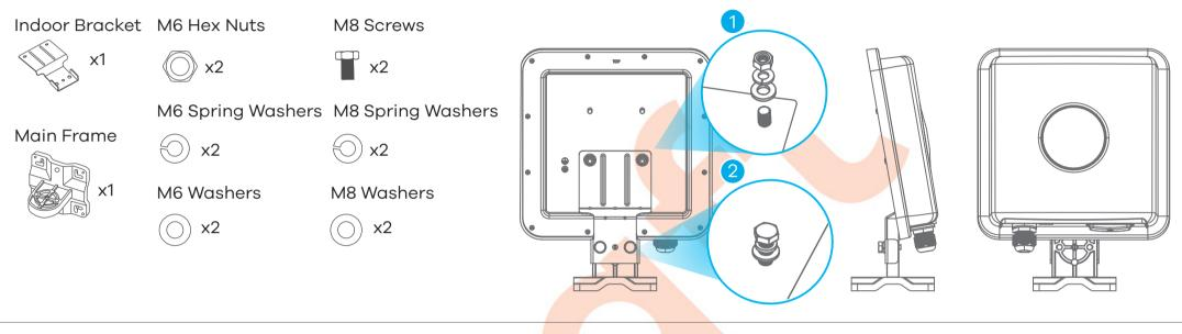
① Use washers, spring washers, and nuts to attach the indoor bracket to the back of the device.
