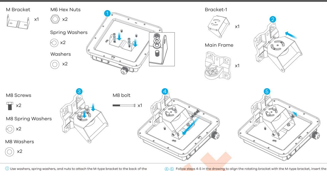
$\bigcirc$  Use washers, spring washers, and nuts to attach the M-type bracket to the back of the LTE7490.
