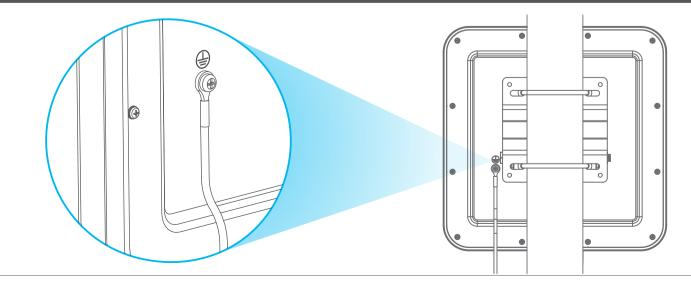
Secure a green/yellow ground cable (18 AWG or smaller) to the LTE7490's rear panel using the M4 ground screw.
