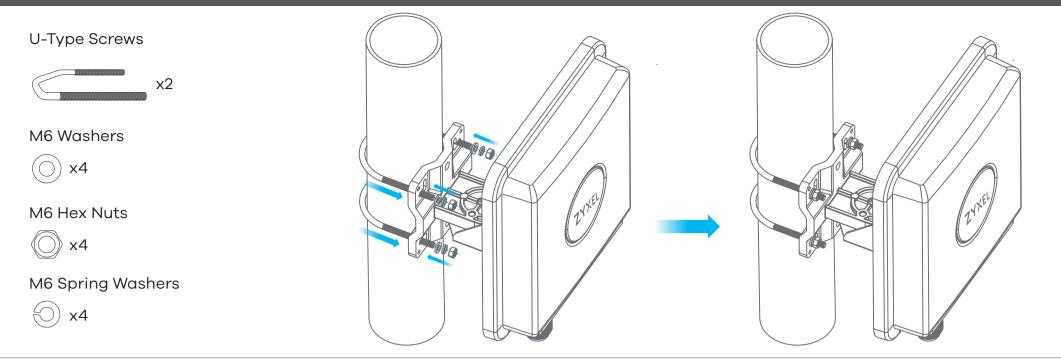
1 Place the U-bolt around a pole. Insert the U-bolt into the holes on the main frame. Use a wrench to secure the main frame to the pole with the washers, spring washers, and nuts.
