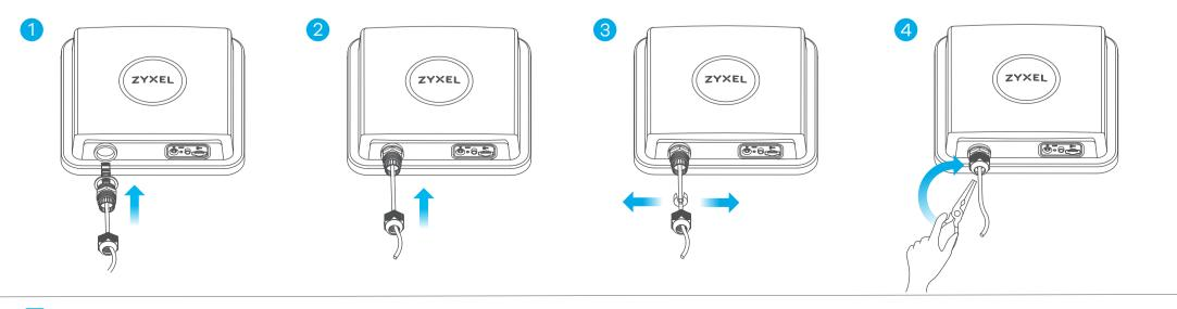
(1-4) Follow steps 1 to 4 in the drawing to connect an 8-pin Cat 5e Ethernet cable to the LTE7490's LAN port.
